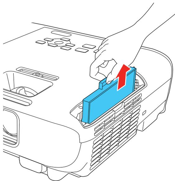
**Note:** Air filters contain ABS resin and polyurethane foam. Dispose of used air filters according to local regulations.
