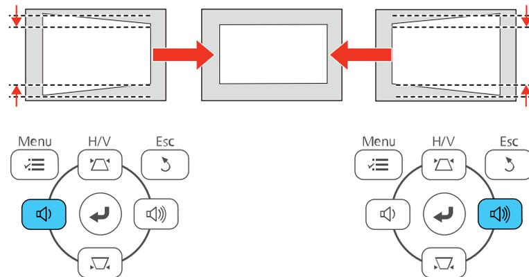
**Note:** The horizontal keystone adjustment buttons are labeled **Wide** and **Tele** on the VS250.
