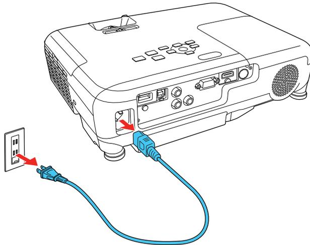
**Caution:** To avoid damaging the projector or lamp, never unplug the power cord when the Status light is on or flashing.
