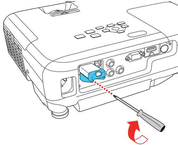
The light on the wireless LAN module turns on when the module is installed and operating. The light flashes when the module is communicating over the network.
