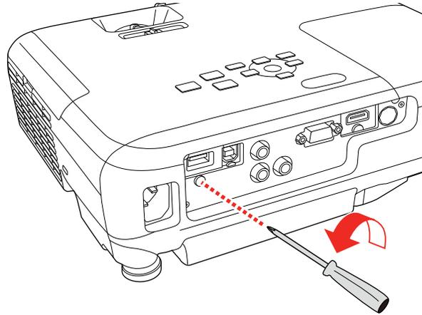
2. Insert the wireless LAN module into the **USB-A** port.
