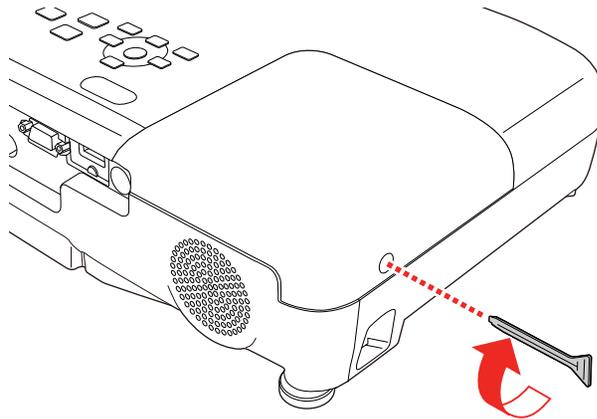
**Note:** Be sure the lamp cover is securely installed or the lamp will not come on.
