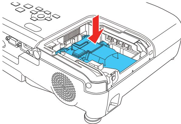
**Caution:** Do not touch any glass on the lamp assembly to avoid premature lamp failure.
