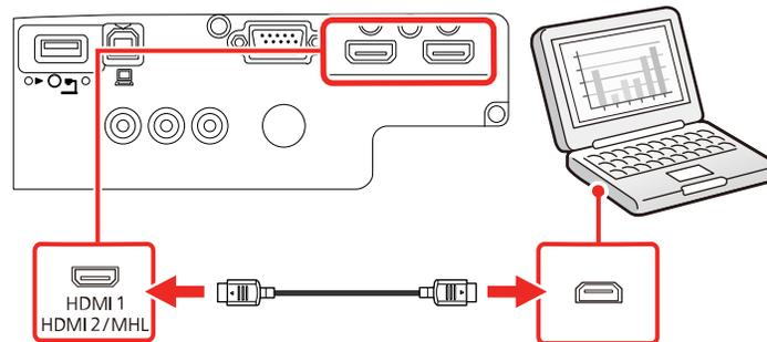
**Note:** The projector converts the digital audio signal sent from your computer into a mono analog signal for the internal speaker.
