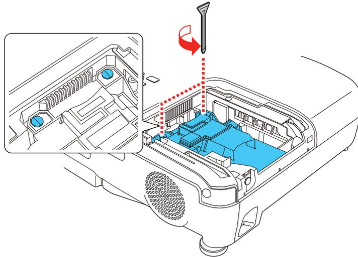
6. Grasp the raised section of the lamp and gently pull the lamp out of the projector.
