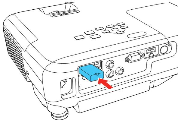
3. Attach the wireless LAN module cover and secure it using the screw you removed.
