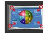
Perfect Fit allows you to make image adjustments by moving the individual corners and sides independent from one another. Ideal for complex installations where sizing screen to image display is more difficult.
