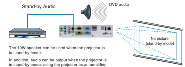
The 10W speaker can be used when the projector is in stand-by mode. In addition, audio can be output when the projector is in stand-by mode, using the projector as an amplifier.
