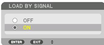
**NOTE:** The Lens Memory function may not produce a completely aligned image (due to tolerances in the lenses) using the adjusted values stored in the projector. After calling up and applying the adjusted values from the Lens Memory function, finely adjust the lens shift, zoom and focus to produce the best possible image.
