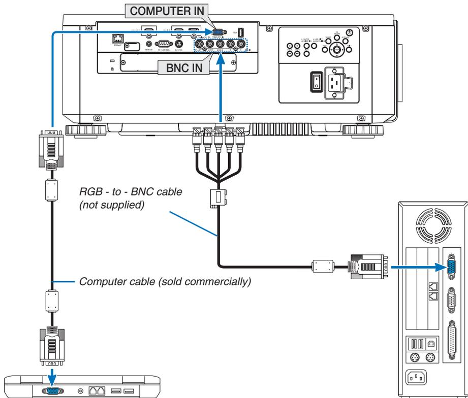
*NOTE: Please check the operating manual of the computer as the name, position and direction of the terminal may differ depending on the computer.*
