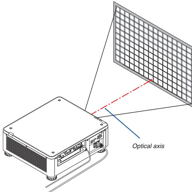
\* When the lens is at the center position, the optical axis is at the center of the image. In this case, adjust the focus at the center of the projected image.
