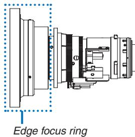
After having removed the lens from the projector and mounted it back, call up the adjusted values stored in the Lens Memory and then follow Step 2 in the procedure above to adjust the focus at the edges of the projected image again.
