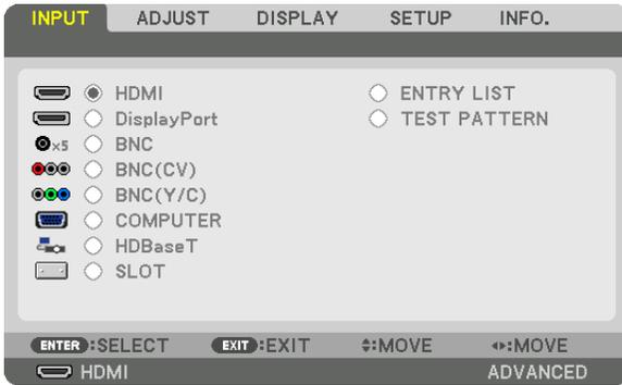
Press the ▼/▲ buttons to match the target input terminal and then press the ENTER button to switch the input. To delete the menu display in the [INPUT] screen, press the MENU or EXIT button.
