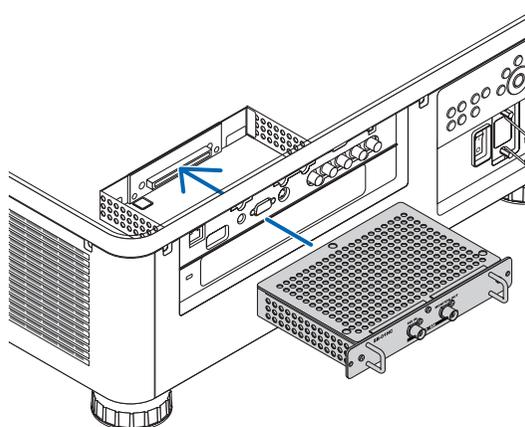
**4. Tighten the two screws on both sides of the slot.**
