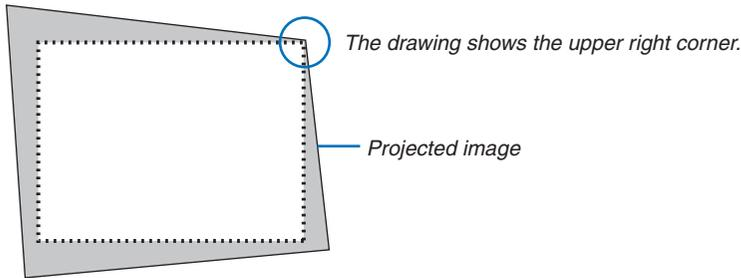
3. **Pick up any one of the corners and align the corner of the image with a corner of the screen.**
