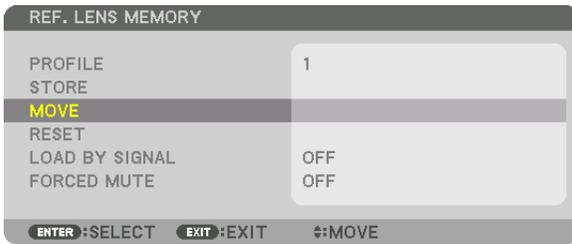
The lens will shift based on the adjusted values stored in the selected [PROFILE].
