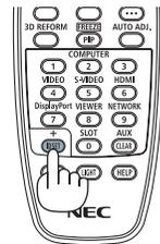
If the projector can be operated with the current remote control ID, the [ACTIVE] will be displayed. If the projector cannot be operated with the current remote control ID, the [INACTIVE] will be displayed. To operate the inactive projector, assign the control ID used for the projector by using the following procedure (Step 3).
