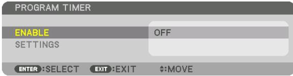
This option turns on/standby the projector and changes video signals, and selects LIGHT mode automatically at a specified time.
