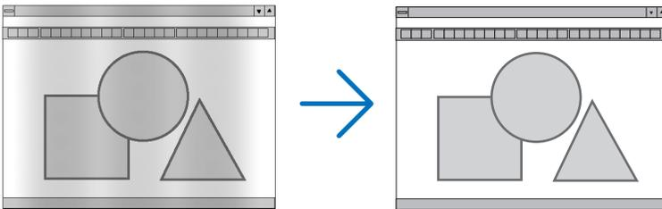
**CLOCK**..... Use this item to fine tune the computer image or to remove any vertical banding that might appear. This function adjusts the clock frequencies that eliminate the horizontal banding in the image.
