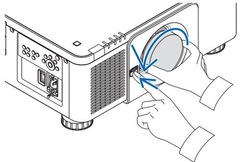
2. After slowly pulling the lens off the projector, release the LENS release button.
