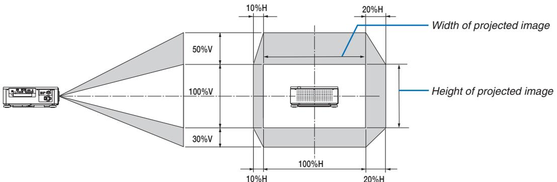
Description of symbols: V indicates vertical (height of the projected image), H indicates horizontal (width of the projected image).
