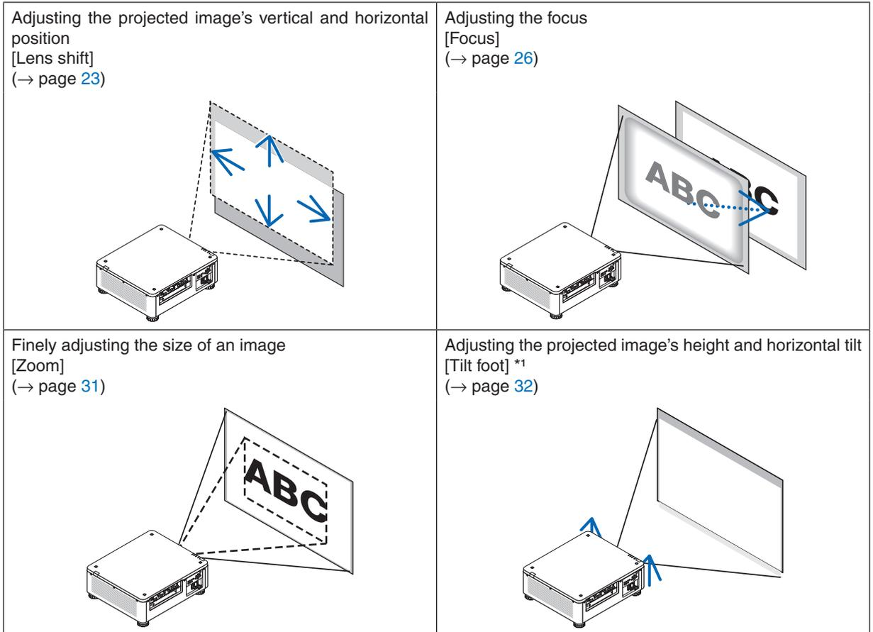
**NOTE\*1:** Adjust the projected image's height using the tilt foot when you want to project the image at a position higher than the lens shift adjustment range.
