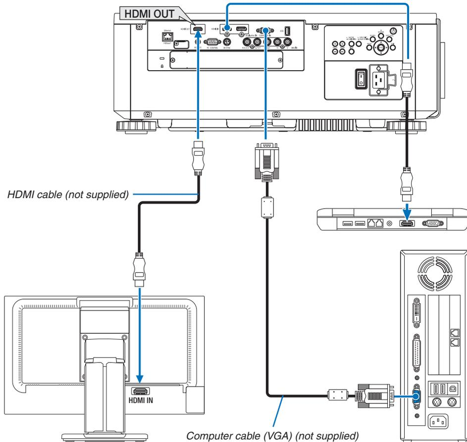
You can connect a separate, external monitor to your projector to simultaneously view on a monitor the computer analog image you're projecting.
