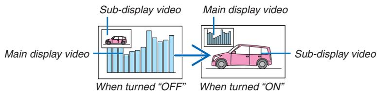
The signal output from the **HDMI OUT** terminal does not change even if the display positions are switched.
