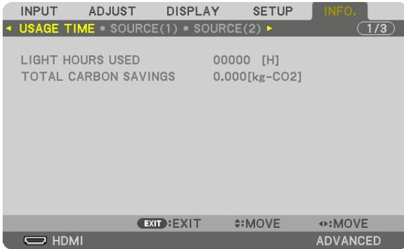
The [CARBON SAVINGS-SESSION] message shows the amount of CO<sub>2</sub> emission reduction between the time of changing to LIGHT MODE immediately after the time of power-on and the time of power-off. The [CARBON SAVINGS-SESSION] message will be displayed in the [POWER OFF/ ARE YOU SURE ?] message at the time of power-off.
