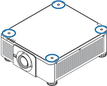
(1) Use your tweezers or nail to pinch and pull up the rubber cap.
