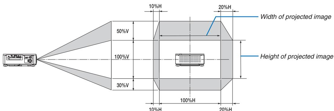
\* The lens shift range is the same for ceiling installation.
